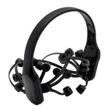
Emotiv EPOC is **a high resolution, multi-channel, wireless neuroheadset**. The EPOC uses a set of 14 sensors plus 2 references to tune into electric signals produced by the brain to detect the user's thoughts, feelings and expressions in real time. The EPOC connects wirelessly to PCs running Windows, Linux, or MAC OS X.
